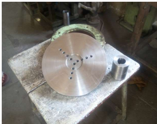
FIGURE 6.4: Disk type crank plate with stroke adjuster hole. (Designed and manufactured for the research experiment)
